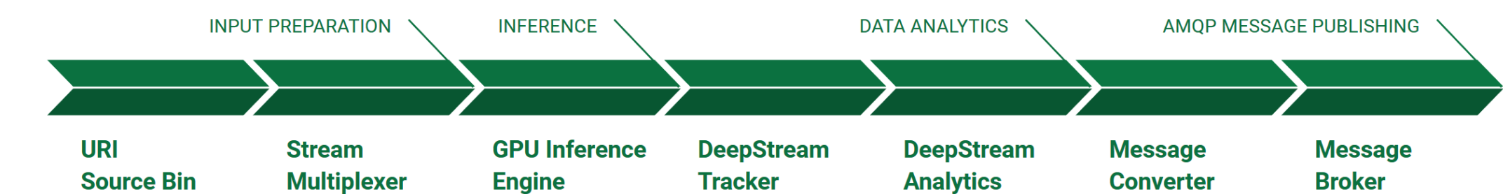
Fig. 2: DeepStream YOLOv3 Application Pipeline
